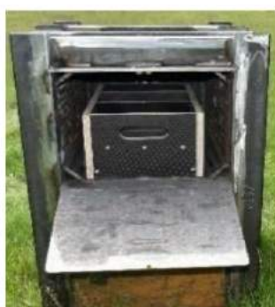
Fig. 3. Arrangement of steel box with stiffening elements and tigo wooden box inside
