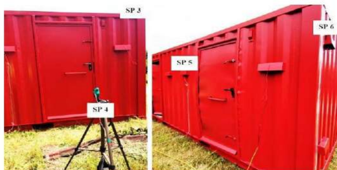
b) Arrangement of the 4 pressure sensors
