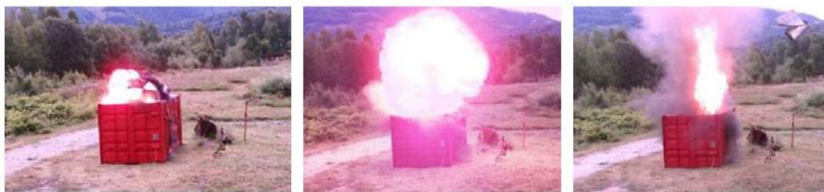
Fig. 10. Visualization of detonation and air shock wave propagation test no. 1
