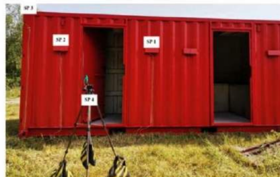
Fig. 9. Container test no. 1 - arrangement of the 4 pressure sensors
