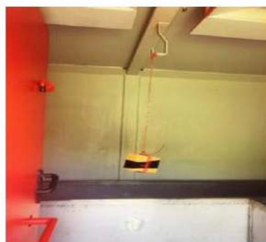
a) Suspended charge of 1.5 kg. TNT
