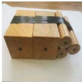
Fig. 8. Location of the explosive charge in compartment no. 1 of container
