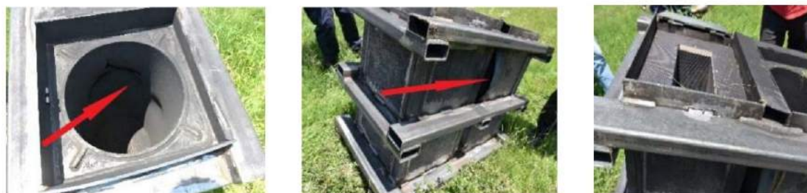
Fig. 6. Effects of testing the steel box with inserted pipe
