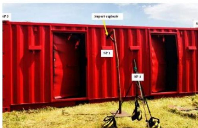
b) Arrangement of the 4 pressure sensors
