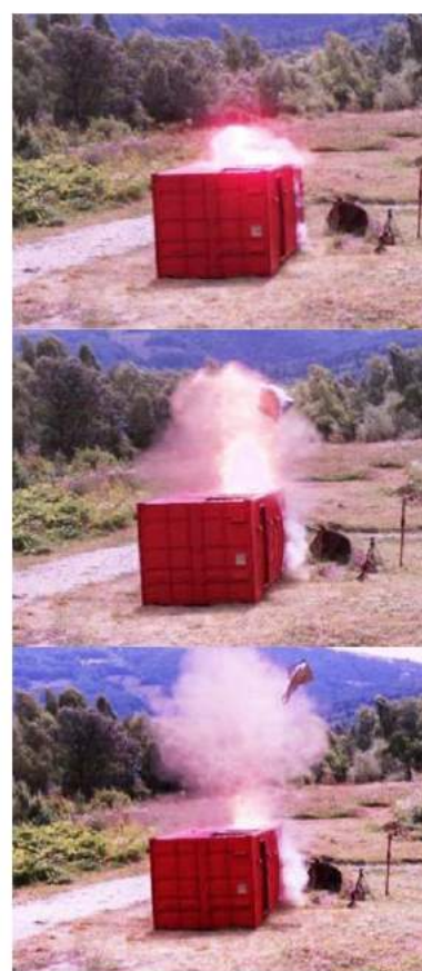
Fig. 14. Visualization of detonation and air shock wave propagation test no. 2
