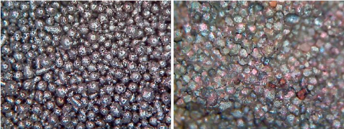
Pic. 16: Stellite granules on steel; left before, right after explosion
