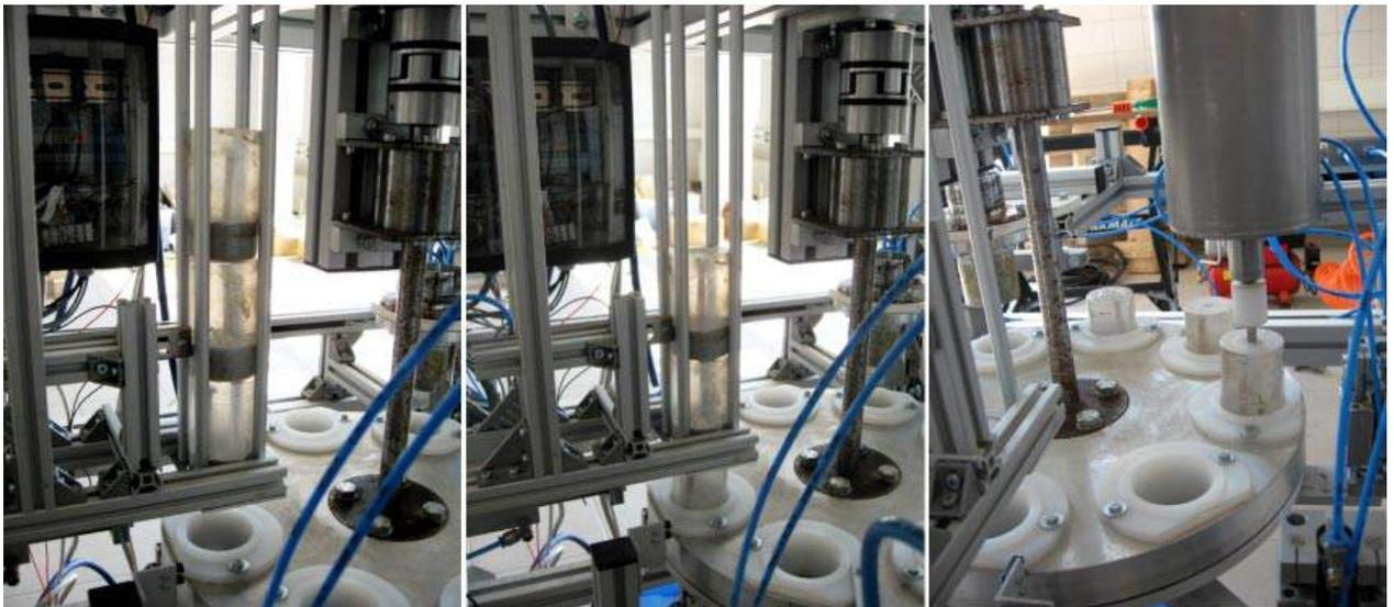
Picture 3 a - c: View of the rotary conveyor of the LOX-Ex filling machine
