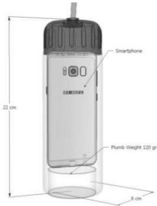
Figure 3. Smartphone used to measure holes
