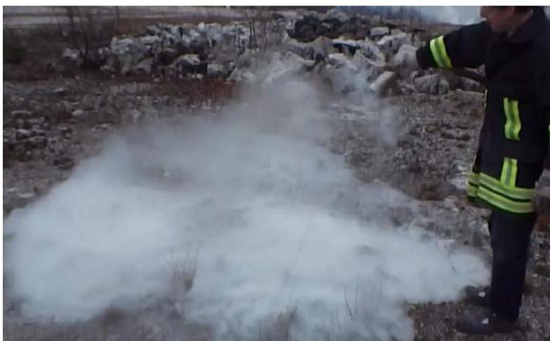
Pic. 5: Disposal of PMMA-LOX-Ex; here approx. 300 g
