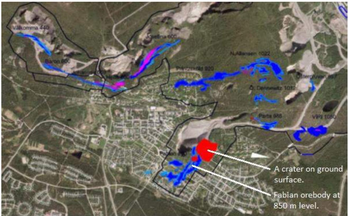
Figure 2. Aerial view of the Malmberget Mine site. Colored objects are horizontal projections of the orebodies at a specific level shown above.
