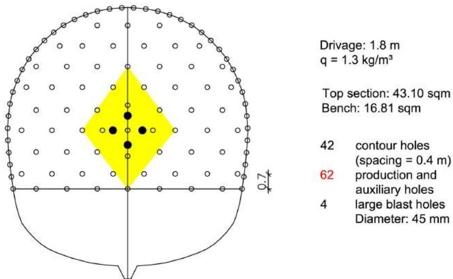
Fig. 15: Drill pattern for drill and blast with a blasting pull of 1.80m and  $q = 1.3 \text{ kg/m}^3$
