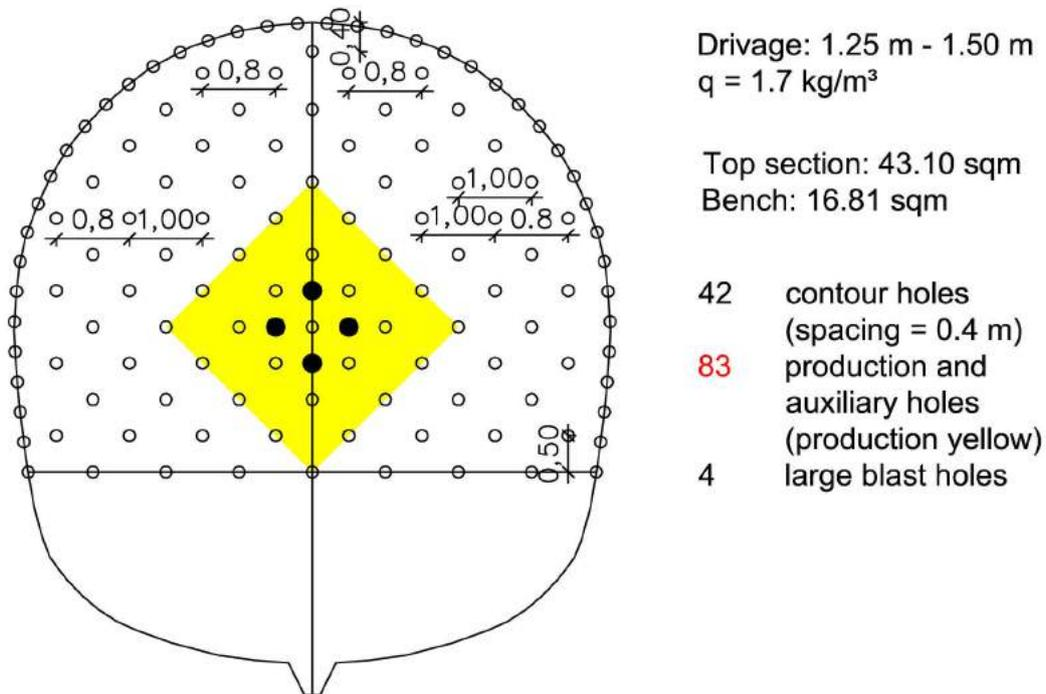
Fig. 14: Drill pattern for drill and blast with a blasting pull of 1.20–1.50m and  $q = 1.7 \text{ kg/m}^3$
