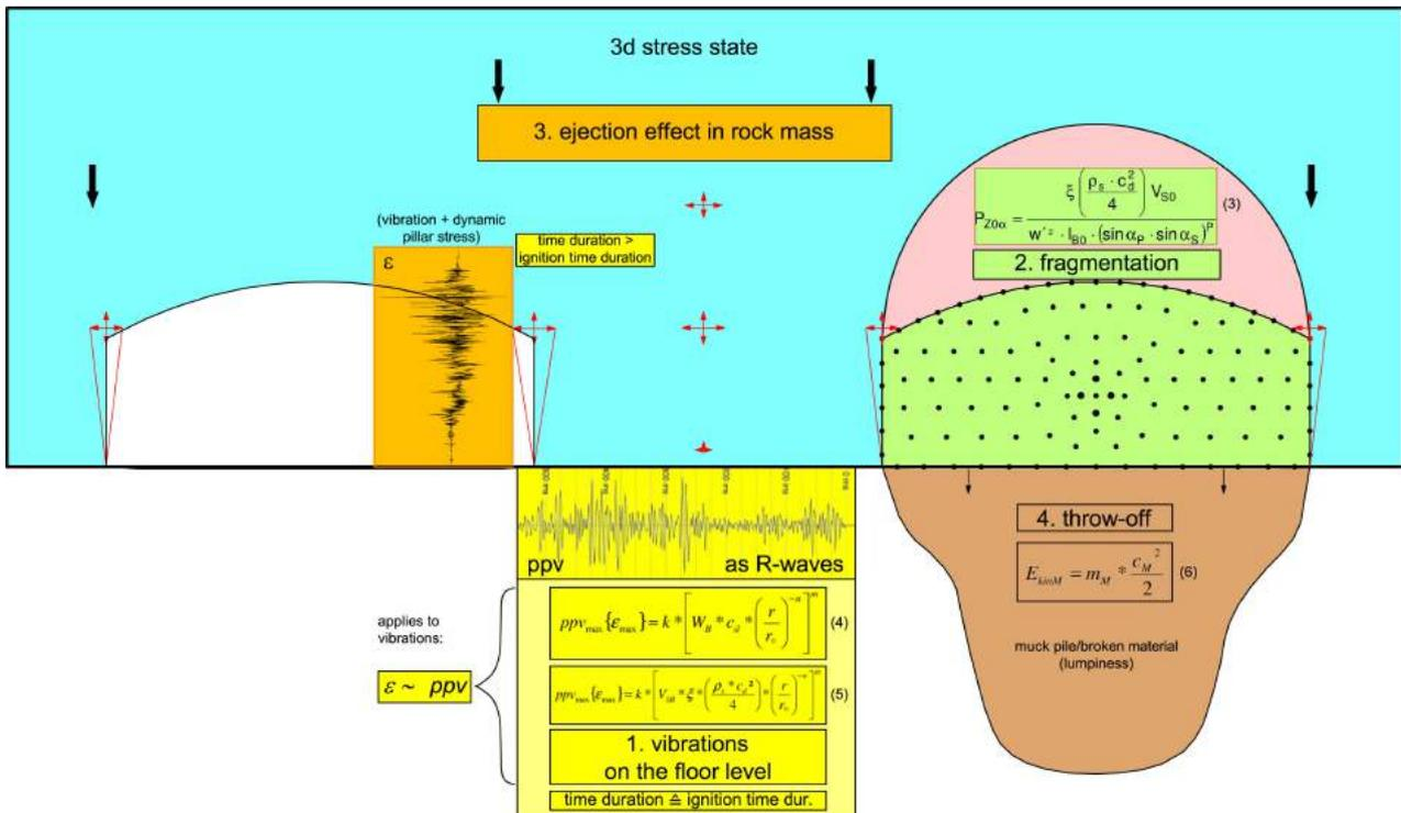
Fig. 12: Four-phase model of 3-D blasting underground
