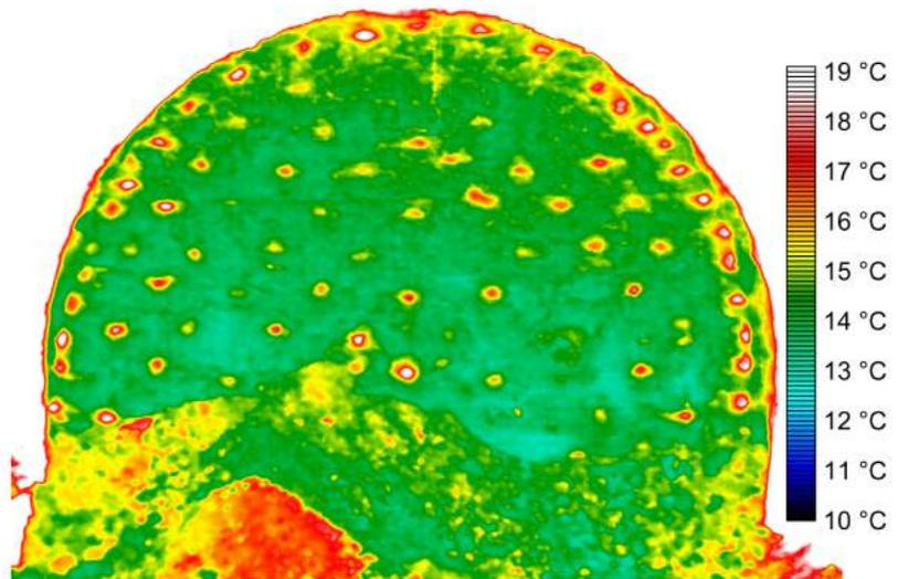
Fig. 27: Thermogram after blasting the roof section showing hot areas near charges detonated in blast holes
