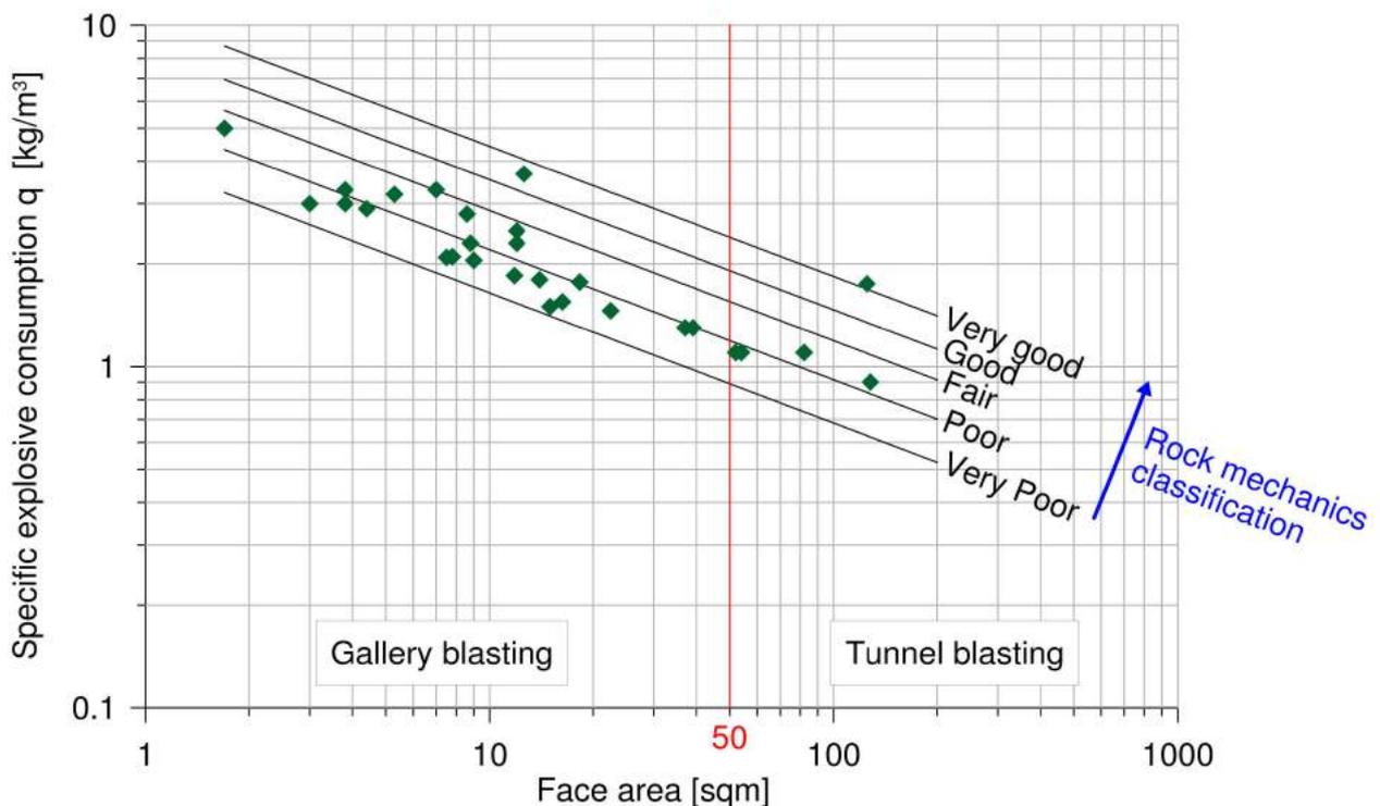
Fig. 13: Graph used to estimate the specific explosive consumption  $q$  (in kg/m<sup>3</sup>) depending on the face area and excavation strength [after 7]
