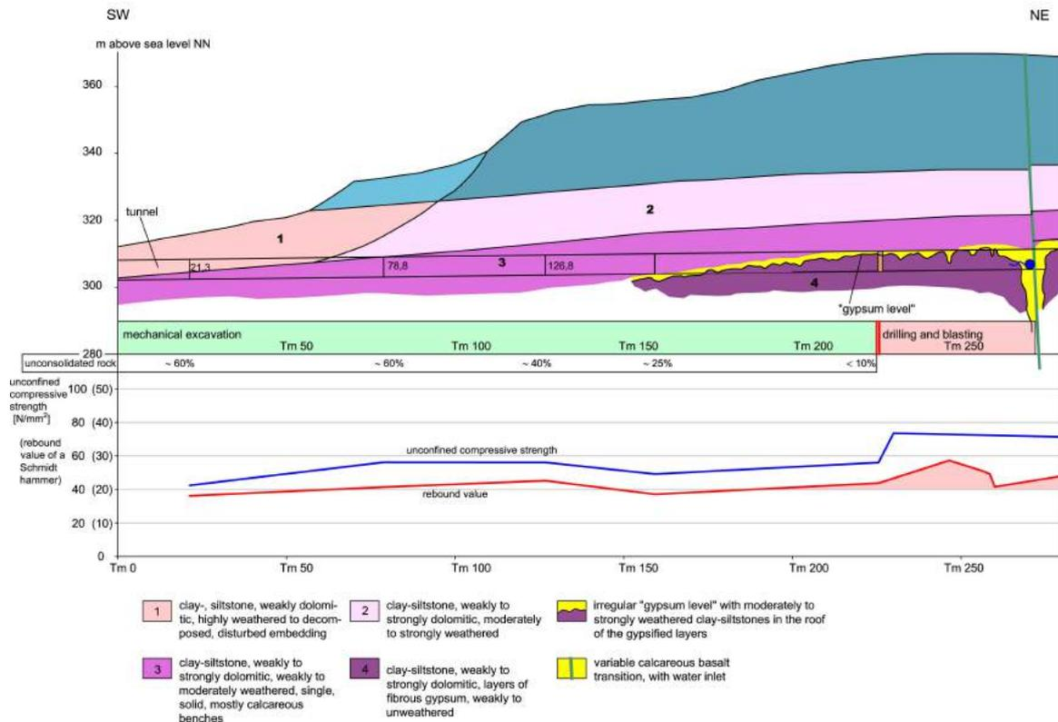
Fig. 4: Extract of the tunnel geology from tunnel metre 0 (west portal) to tunnel metre 280
