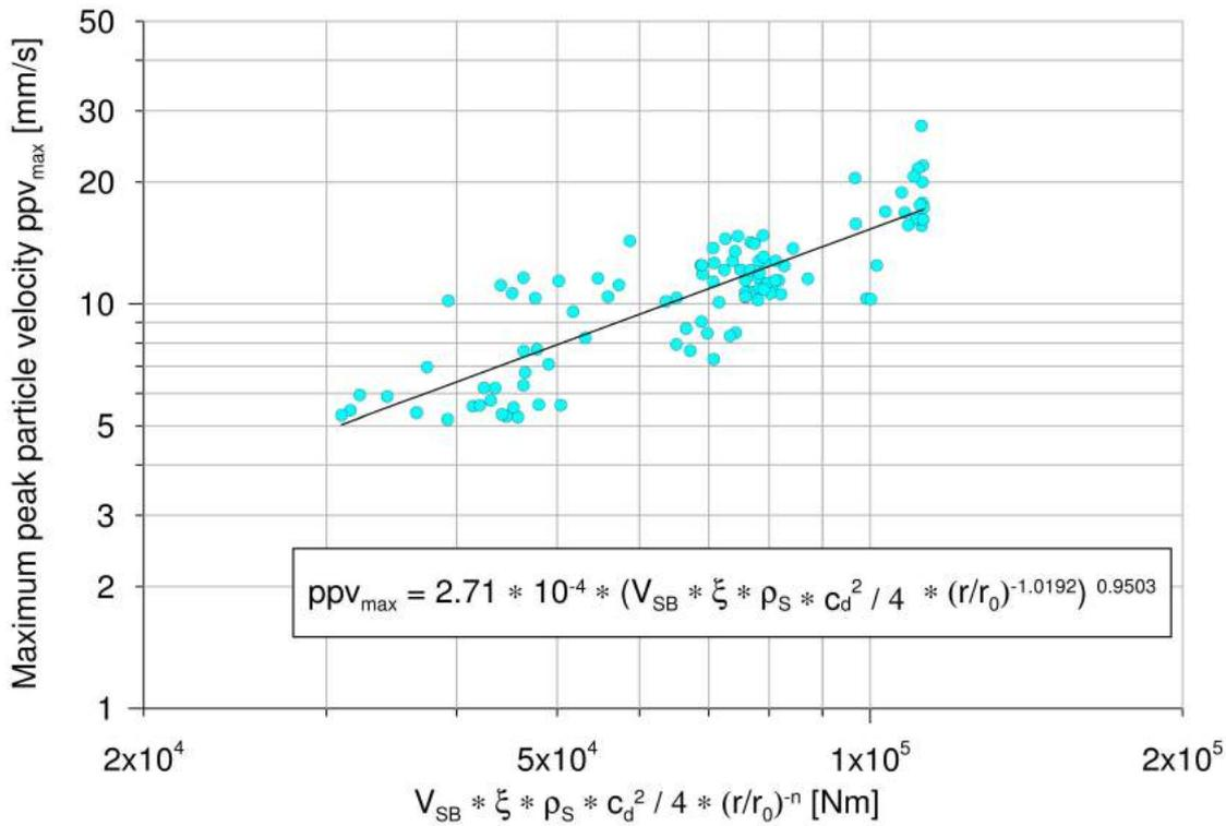
Fig. 23: Theoretical energy-distance correlation from tunnelling in Zierenberg with transonic effect due to the high velocities of the rock in situ
