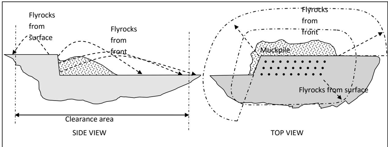
Figure 3: Zones affected by flyrock resulting from blasting
