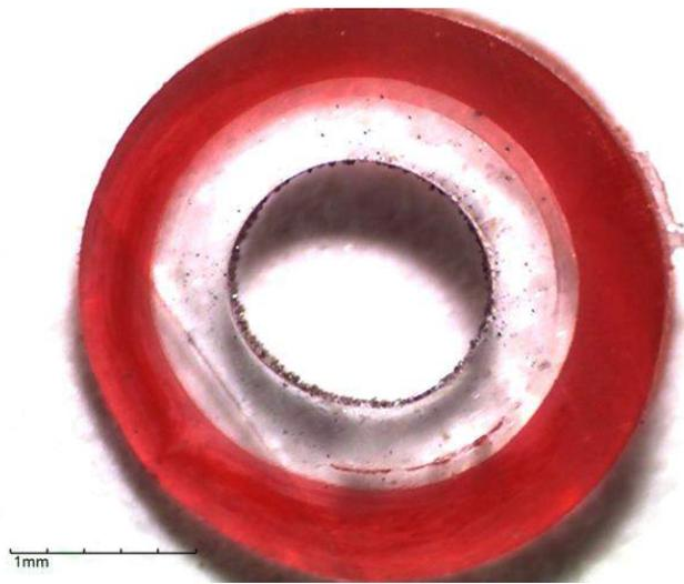
a) optical 3 mm shock tube cross section
