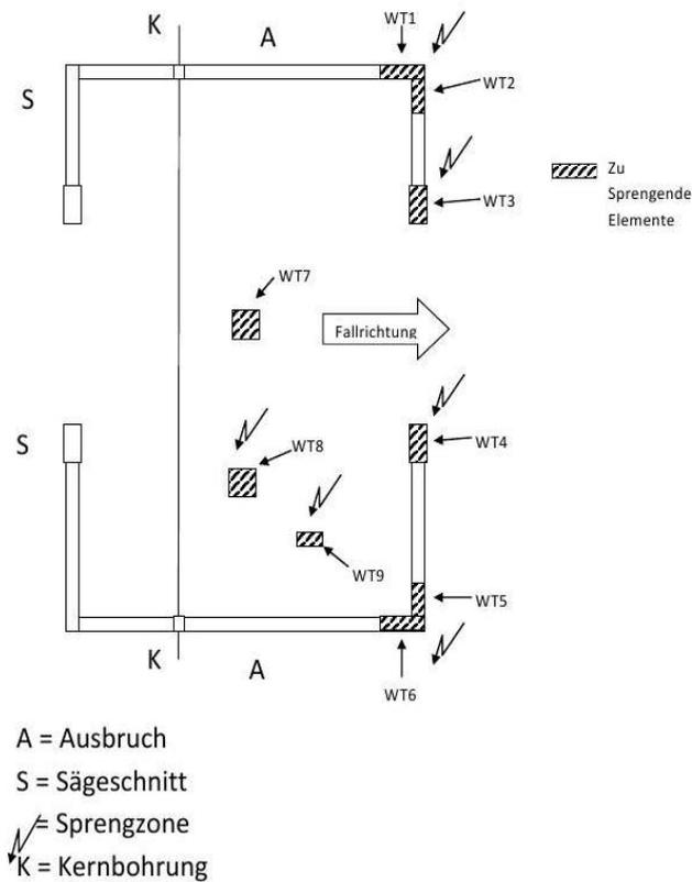
The blasting mouth is formed directly by the walls and the pillars. WT1--WT9. The walls in the falling direction are demolished to a height of 8 m and the pillars in the interior to a height of 4.80 m. All drilling operations were done with Tamrock Commando 100 and 120 using a drill hole diameter of 36 millimeters. All examined drill holes were marked yellow;; all holes to be drilled or drilled again were marked with red colour.
