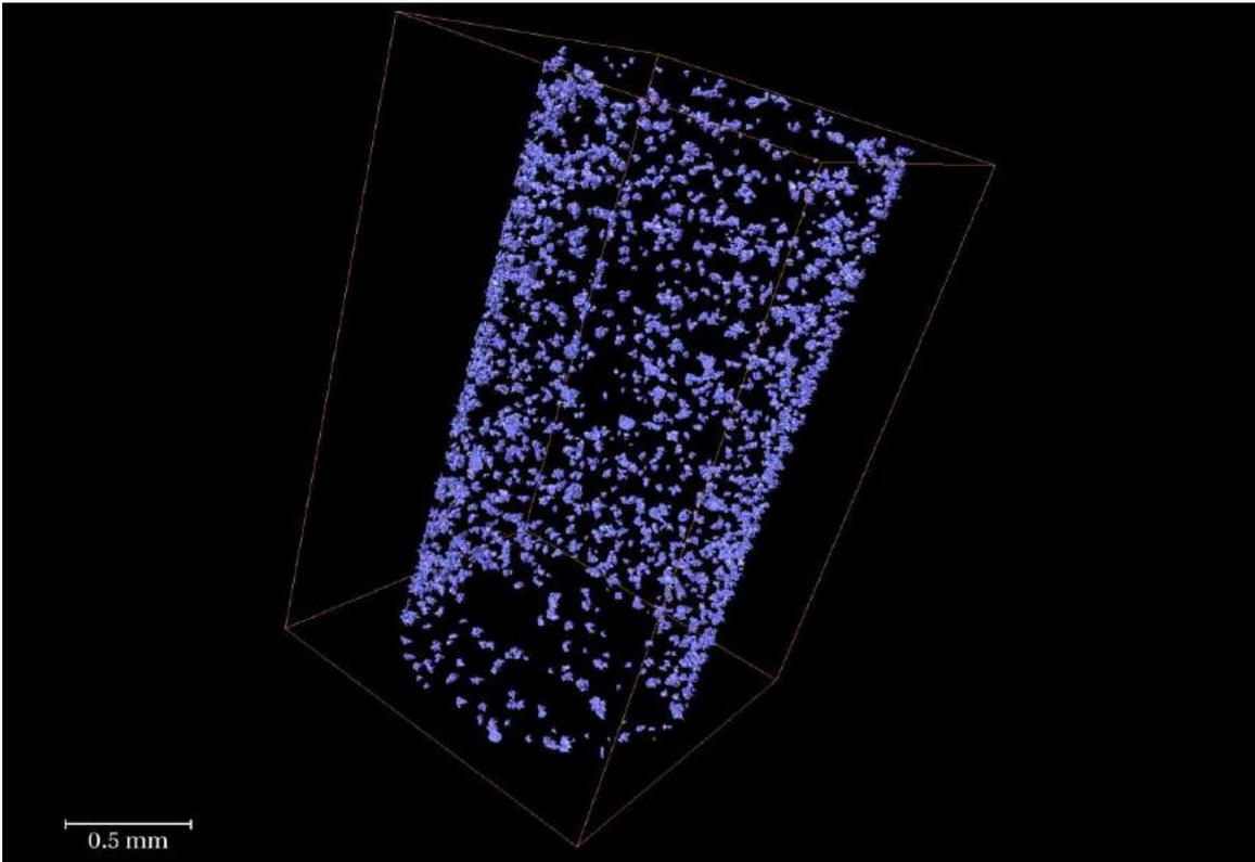
Figure 3: 3D rendering of explosive particules showing particle distribution.
