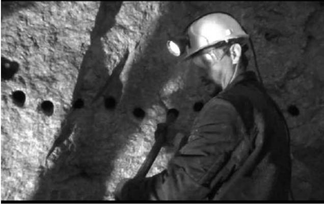
Picture no. 9 - Loading of boreholes
