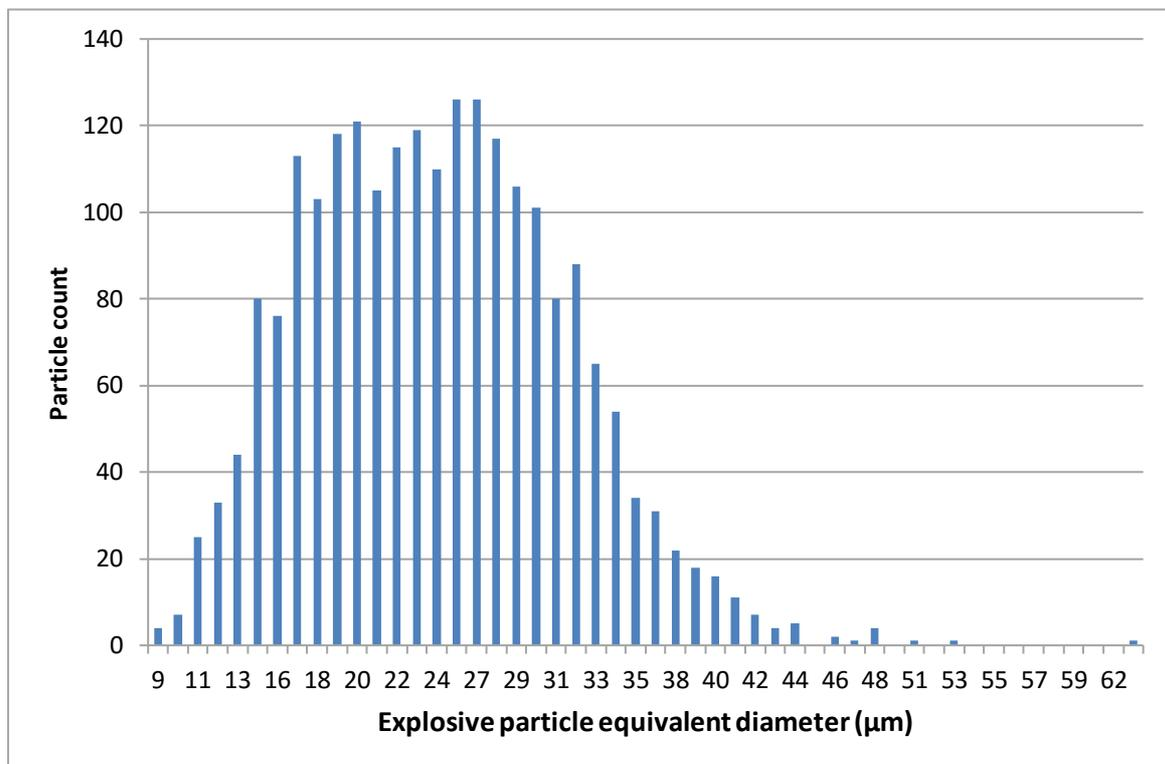
Figure 4: explosive particle size distribution.
