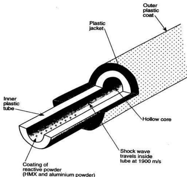
b) schematic of shock tube, from [2]
