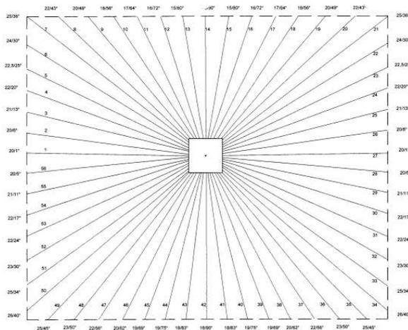
Picture no. 4 - South chimney drilling pattern
