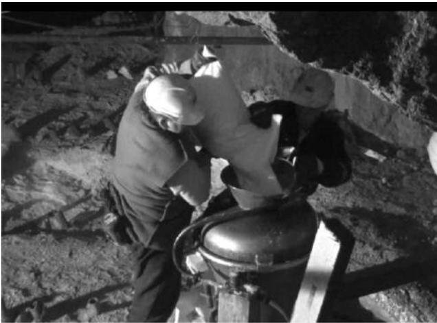
Picture no. 10 - Completing of explosive into the loading device
