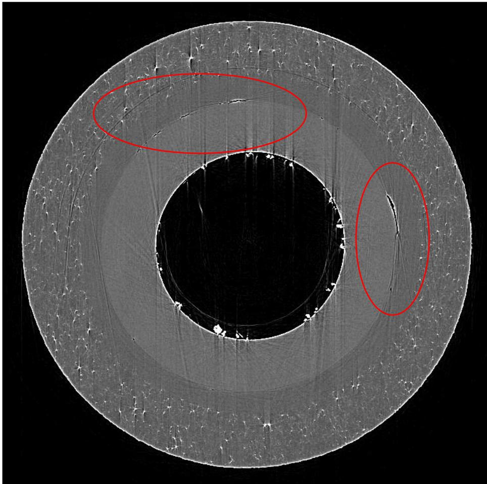
Figure 2: Examples of defects (cracks) on a 2D CT slice.
