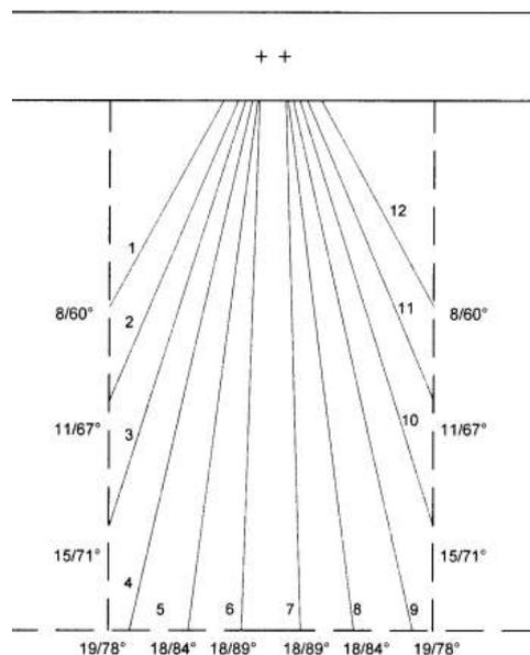
Picture no. 6 - Liquidation gangway drilling pattern
